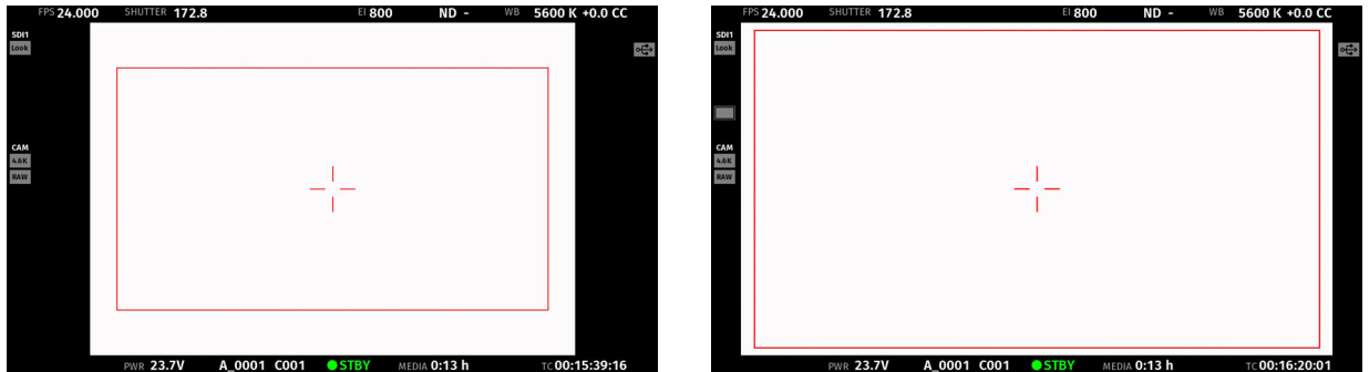
Two screen grabs from an ALEXA 35 in sensor mode 4.6K 3:2 Open Gate with a custom 16:9 4K frame line (red rectangle) applied. The left screen shot shows the SDI 1 output without magnification applied. The right screen grab shows the SDI 1 output with magnification applied to enlarge the image (in this example set to 130%).
